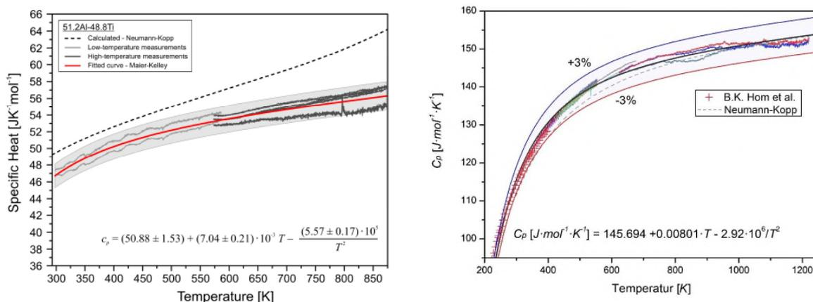
Fig. 1: Heat capacity measurements of the intermetallic  $\gamma\text{-TiAl}$  phase (left) [1], and the ceramic compound  $\text{ZrTiO}_4$  (right) [2].
