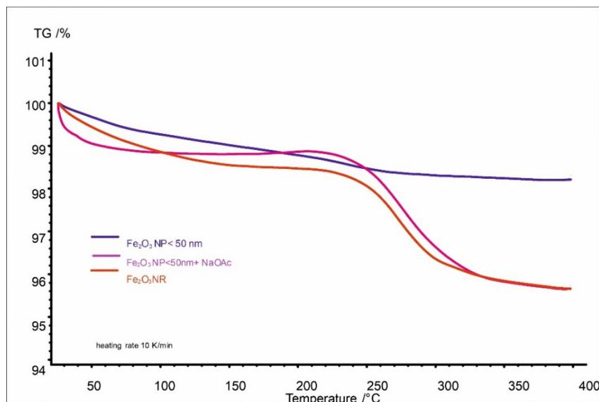
**Figure 1:** TG measurement of the  $\text{Fe}_2\text{O}_3$  nanorods ( $\text{Fe}_2\text{O}_3\text{NR}$ ) and the commercially purchased hematite nanoparticle with ( $\text{Fe}_2\text{O}_3\text{NP}<50\text{nm}+\text{NaOAc}$ ) and without ( $\text{Fe}_2\text{O}_3\text{NP}<50\text{nm}$ ) sodium acetate treatment.
