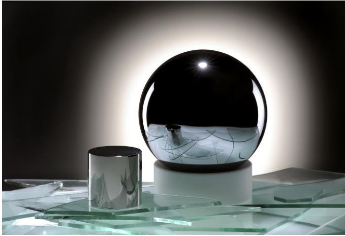
fig. 1 national Pt-Ir kilogram prototype and ^{28}\text{Si} single crystal sphere
