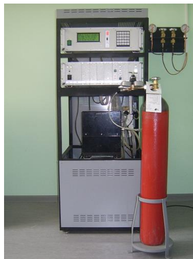
Figure 1 – The Reference Calorimeter System (CAPG / CLCG)
