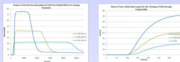
Methylethanolamine (MEA) was added to water in 30% concentration by weight  $\text{CO}_2$  absorption was monitored at three different flow rates.
