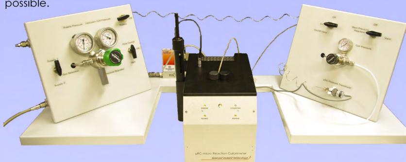
The option has been used to good effect to study Carbon Capture involving the exothermic reaction that occurs when  $\text{CO}_2$  gas is absorbed by an amine solution. The GFO consists of a flow controller to regulate the flow rate of  $\text{CO}_2$  into the cell containing the amine solution. Weighing the vial before and after the test is used to calculate the rate of  $\text{CO}_2$  uptake.
