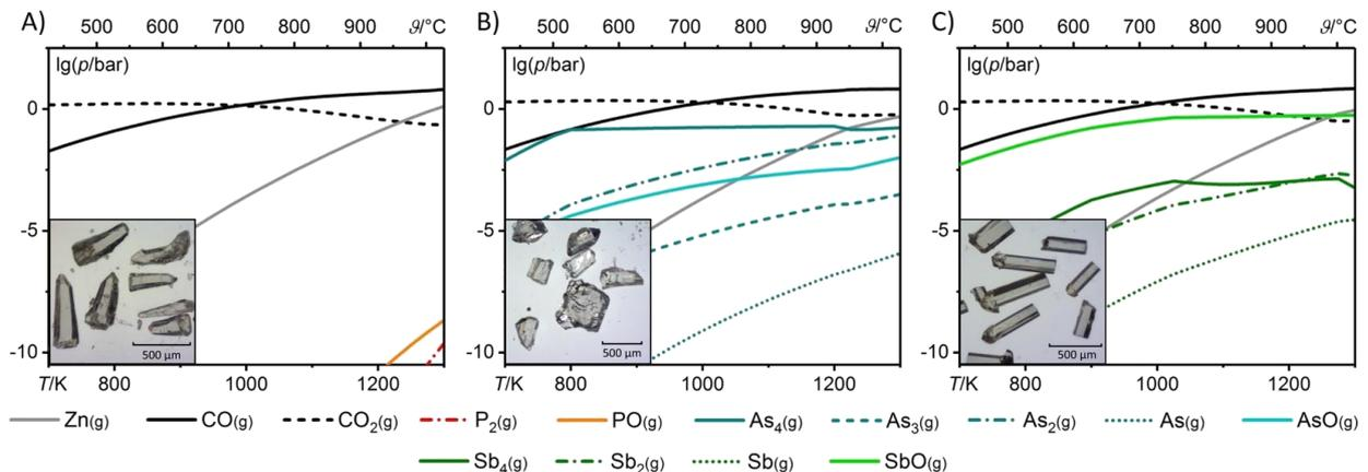
**Figure 1:** Composition of the gas phase, calculated by TRAGMIN and ZnO crystals grown by CVT for initial mixtures of zinc oxide, zinc oxalate, graphite, and addition of: A) phosphorus, B) arsenic, C) antimony
